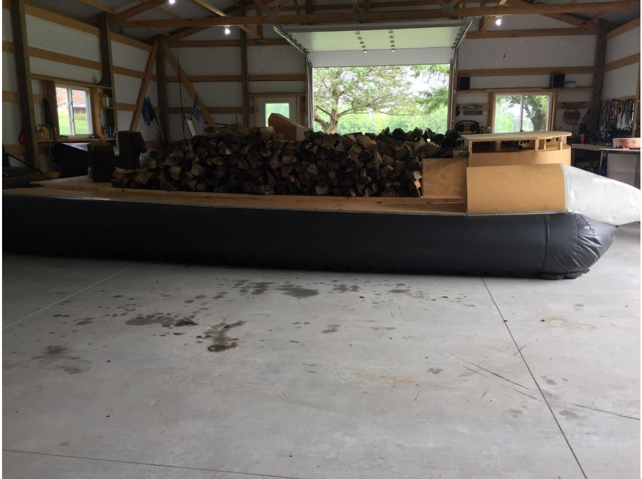
The Hovertoon test plat floating with 5000 pounds of weight to test the motor, centrifugal clutch, belt, centrifugal fans, and skirt.
