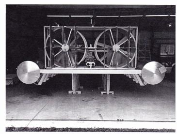
By the end of August, the first water tests were completed. and some modifications were needed for the skirt. The problems being there were no anti-scoop flaps in the rear and the bag to lift vents were in the center and not as a feed to each finger. Once those two things were corrected, the craft performed very well. By October, confidence was to the point where a 10-mile trip was taken with no chase boat.
