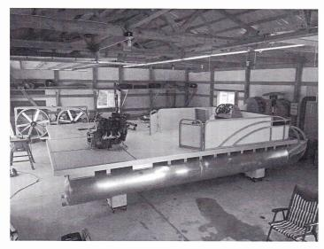
With the above done, the skirt sections were ready to be added. The 18-ounce per yard bag skirt comes in 4 pieces; front, rear, and the 2 sides which are all zipped together and connected to the craft using awning rail supplied from Oshkosh Tent and Awning. There are zippers on finger sections for each of the bag sections, then tie wraps are used to keep everything from un-zipping.
