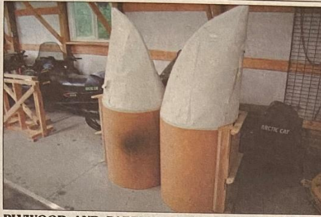
PLYWOOD AND PARTICLE board were used for the fake front ends on Richard Schramer's Hovertoon test platform.
